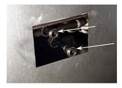
Figure 5. Oil return and rinse-line (where applicable) connections.
